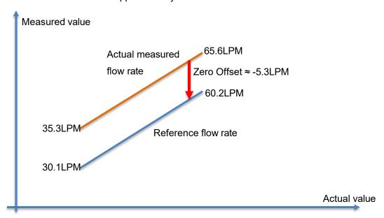
Press and hold the confirmation button  $\rightarrow$  Settings  $\rightarrow$  Flow Measurement  $\rightarrow$  Zero Offset  $\rightarrow$  Set the offset value to -5.3LPM (default value is 0) to complete the offset configuration.
