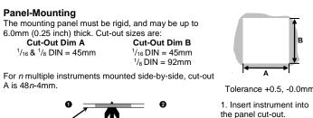
2. Hold front bezel firmly (without pressing on display area), and re-fit mounting clamp. Push clamp forward, using a tool if necessary, until gasket is compressed and instrument held firmly
