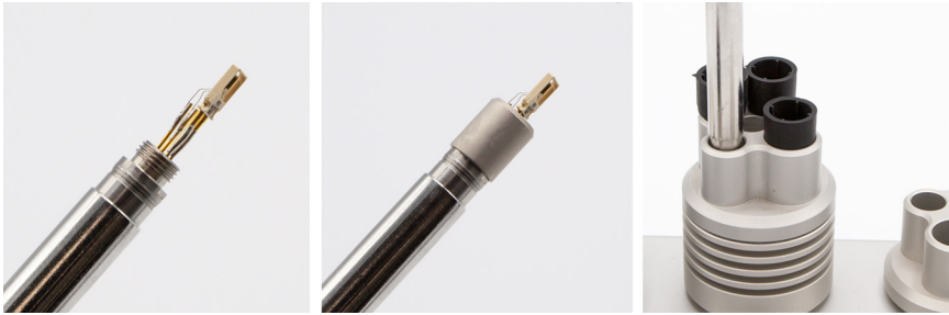
Figure 30 HMP5 calibration with HMK15 using 211302SP adapter
