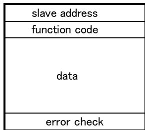
2) Communication command format (MODBUS: Described by RTU because RTU is foundation)
