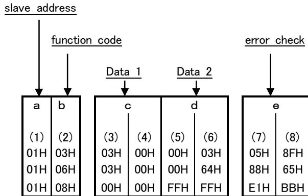
3) Communication answer format (MODBUS: Described by RTU because RTU is foundations)
