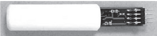
Replaceable Sensor with Sintered Filter
