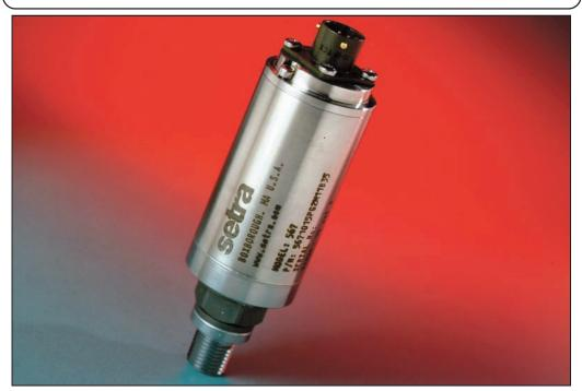
etra's Model 567 high performance pressure transducer offers customer accessible down-ranging capabilities, making this unit ideal for high overpressure applications. The 5:1 turndown is easily accessed via a switch and potentiometer.
