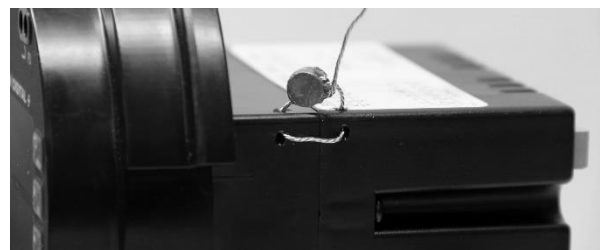
Figure 6: Close and Crimp Seal Wire Security Loop
