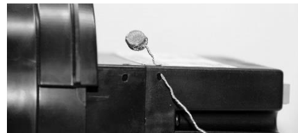
Figure 4: Wire Loop through Rear Case Pass-Through
