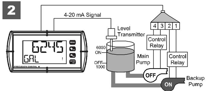
3. If the backup pump is not able to keep up, and the level reaches 7000 gallons, relay #2 transfers and starts the main pump as well.
