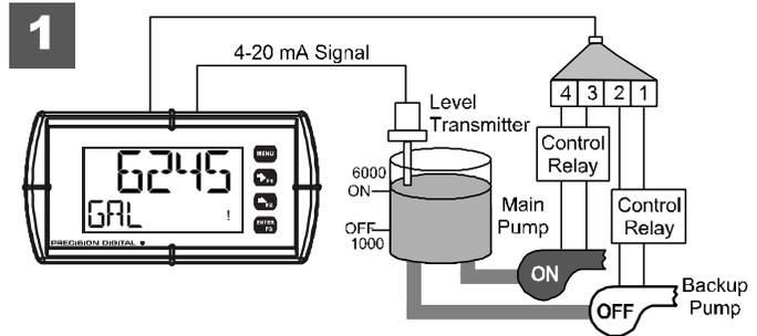
2. With the Pump Alternation feature activated, the next time the level reaches 6000 gallons, relay #1 transfers and starts the backup pump.
