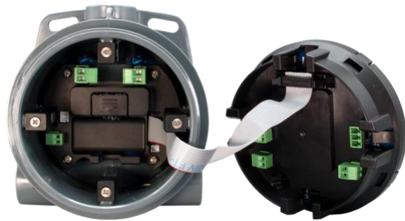
Options Board Connected to Display Module
