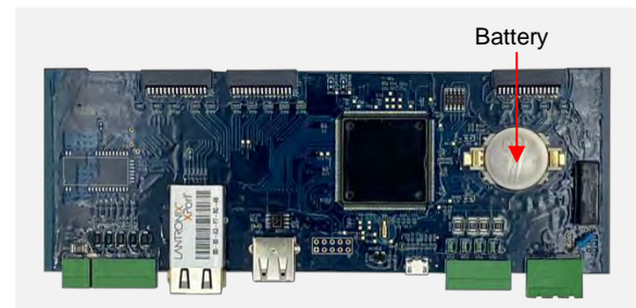
Main MCU Board Showing Battery Location
