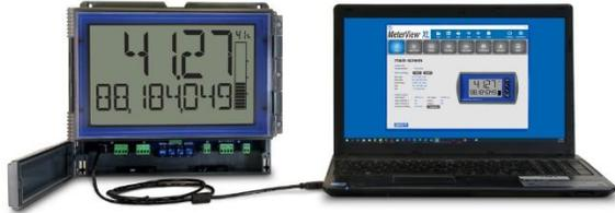
Free, PC-based, MeterView XL software that connects to the meter via a USB cable is available for programming and setup of the meters. This software greatly simplifies the programming process and allows the user to save configuration files for later use. The meter will also be powered by the USB connection so no additional power is needed during programming.
