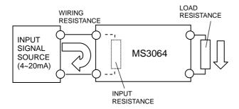
Note: The input resistance for the voltage output model is fixed to approx.  $250\Omega$  (for 20mA DC input).
