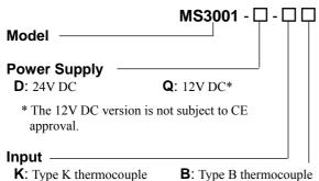
**K**: Type K thermocouple **E**: Type E thermocouple **J**: Type J thermocouple **T**: Type T thermocouple
