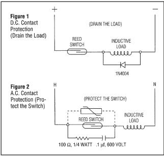
Note: Max. Leakage Current: 4ma @ 120 VAC
