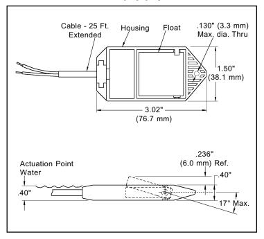
The LS-10's rounded design makes it easy to remove for cleaning and reinstall after an alarm condition is triggered, or for maintenance.
