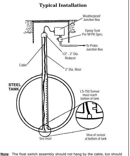
rest lightly on the bottom of the tank supported by the cable.
