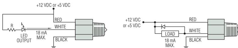
Note: Inductive loads must be diode suppressed.
