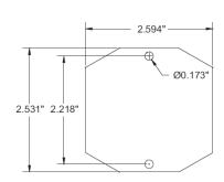
Mount the octal socket (base) on rigid vertical or horizontal surface using #6 or #8 screws. The control should be mounted within an enclosure of proper NEMA integrity.
