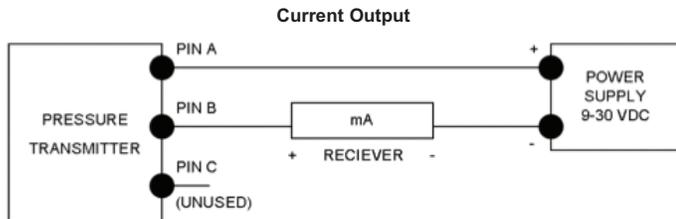
Figure B: Current Output Connection
