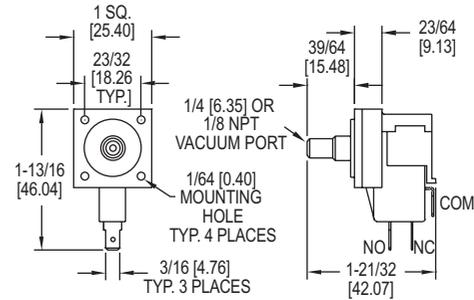
Compact, lightweight, and adjustable, the **Series MVS Miniature Vacuum Switch** is specially designed for OEM applications. This low cost switch has a minimum life expectancy of 10 million cycles and has an extremely fast response time. Typical applications for the MVS are HVAC, home appliance, dairy systems, medical, office equipment, and pump control.
