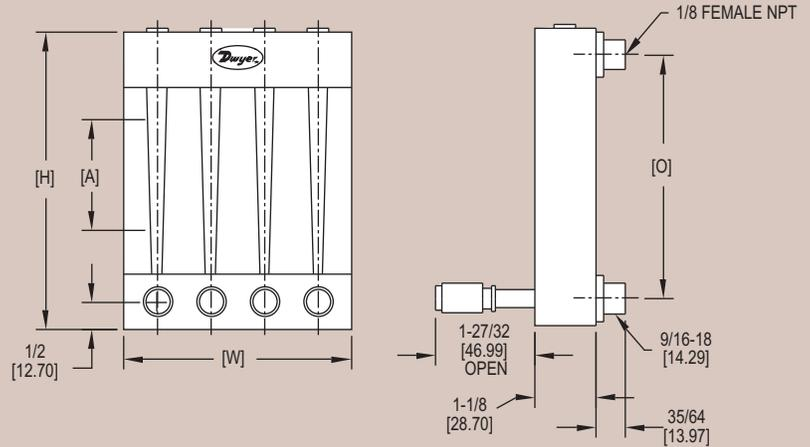
**Customize flow systems** to meet application requirements. Systems can be configured with up to six different flow tubes with various flow capacities and flow patterns. The Series MTF Multitube Flow Systems are ideal for multichannel metering, mixing, or monitoring applications.
