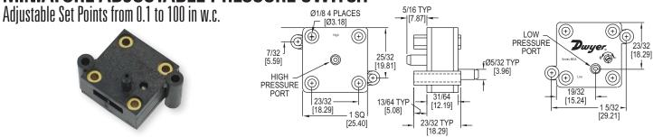
Series MDA Miniature Adjustable Pressure Switch is used to sense differential pressure. The switch features field adjustable set point and gold inlay contacts. Air or other compatible fluids can be used on the "high side". The lightweight and compact size make the MDA ideal for any application with space constraints. Applications include industrial, HVAC, pump and motor control, medical, automotive, pools and spas.
