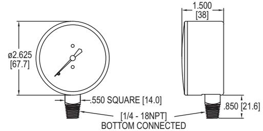
Our **Series LPG4 2.5" Low Pressure Gage** offers top of the line performance and accuracy for pressure and vacuum applications up to and including 160 in. w.c. The LPG4 is constructed from a single beryllium-copper diaphragm affixed to a precision-machined brass plate. This innovative design, together with a high-precision, milled-teeth brass movement and nickel-silver pinion and bearing surface, provide the user with a top of the line low pressure instrument.
