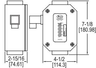
The **Series HFT In-Line Flow Transmitter** provides continuous monitoring of flow rate levels via a direct reading in-line flowmeter with electronics to provide proportional 4-20 mA, 0-5 and 1-5 VDC analog outputs.
