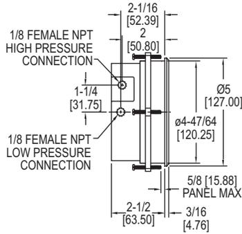
[4] 6-32 HOLES EQUALLY SPACED ON A 5-1/8 [130.18] B.C. PANEL MOUNTING
