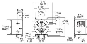
The Series AT22000 ATEX/IECEx Approved Series 2000 Magnehelic<sup>®</sup> Differential Pressure Gage combines the popular Magnehelic<sup>®</sup> line with a flameproof enclosure to extend usage to hazardous locations. This gage can indicate positive, negative or differential pressures and is accurate within 2%
