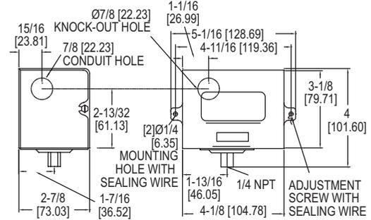
Reliable and convenient, the **Series AP Diaphragm Operated Pressure Switch** is a compact switch for instrument air or other low pressure applications. Visible set point and external adjustment add convenience. Used on air, non-corrosive gas or liquid service compatible with wetted parts. Units are available in weather-proof and explosion-proof housing.
