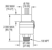
Miniature Series APS/AVS Adjustable Pressure Switch offers reliable switching for pressure/vacuum alarm, shutdown or control. The units are readily adjustable throughout their range using the locking adjusting ring and indicating pointer. The body is constructed of stainless steel for durability in harsh environments. Switches include 12" (30 cm) wire leads sealed with epoxy for additional protection.
