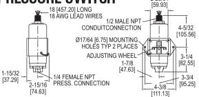
The Series 1000E Explosion-Proof Diaphragm Operated Pressure Switch has the same rugged construction as used in Series 1000W plus explosion-proof design are combined in this new unit. UL listed for Class I, Groups A, B, C & D; Class II, Groups E, F & G. Bellville spring movement permits mounting of control in any position and helps prevent contact chatter. High over-pressure protection and vibration resistance are also featured.
