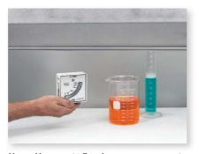
Use a Vaneometer™ swing vane anemometer to measure velocity of air flow into laboratory fume hoods and at paint spray booths to determine when to change filters. Or wherever needed to meet OSHA standards of ventilation for smoke, dust or fume removal.
