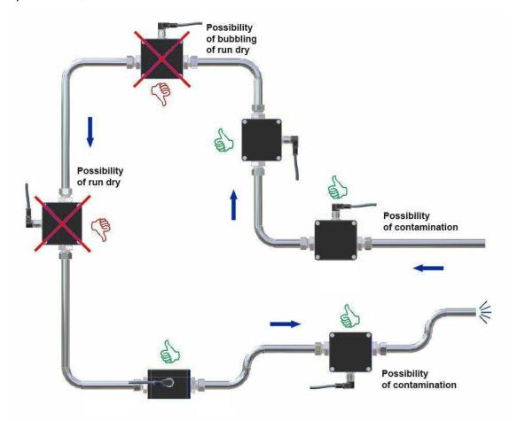
• Installation can occur in horizontal and vertical pipes. The flow sensor is only suitable for application in completely filled pipe systems.
