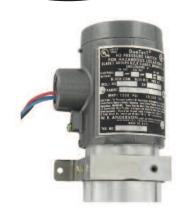
Series H3 Differential Pressure Switches actuate one or two single pole, double throw (SPDT) snap switches in response to increasing or decreasing pressure of compatible gases or liquids. Four field adjustable operating ranges are available allowing set-points up to 200 psid. All models are suitable for hazardous locations and also include weatherproof housings as detailed in the chart below. Read and understand instructions completely before proceeding with installation or operation.
