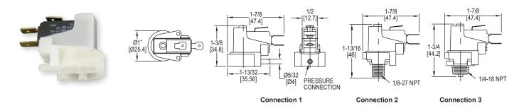
Series A7 Mini Pressure Switch has been designed for high current applications. These switches are small and inexpensive, making them ideal for OEM use. The Series A7 switches utilize a high-quality snap-action switch, which is diaphragm actuated. They have a silicone diaphragm and nylon housing. The A7 switches are compact and lightweight which adds to the ease of installation. The set point must be factory set, but a broad operating range makes them great for a variety of applications.
