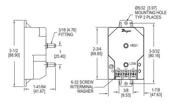
Our low cost Series 668 Differential Pressure Transmitter is capable of measuring low pressures with a ±1% accuracy ideally suited for proper building pressurization and air flow control. Transmitters can withstand up to 10 psig overpressure with no damage to the unit. Variable capacitance sensor design provides excellent sensitivity and long-term stability. Compact, lightweight design makes installation simple and easy. Units also feature reverse-polarity protection.
