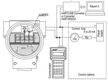
Figure 3a: The link of transmitter and communicator or converter to current line by the control cabinet throughout
