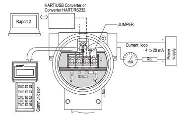
Rys. 2b Figure 3b: The link of transmitter and communicator or converter to <SIGNAL+> <SIGNAL-> transmitter terminals in case of the resistance in current loop is higher than  $240\Omega$
