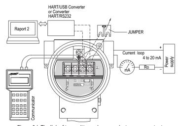
Figure 3d: The link of transmitter and communicator or converter to <SIGNAL+> <SIGNAL-> transmitter terminals in case of the resistance in current loop is smaller than 240 $\Omega$
