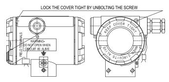
Figure 6: How to lead the casing of Series 3500 transmitters
