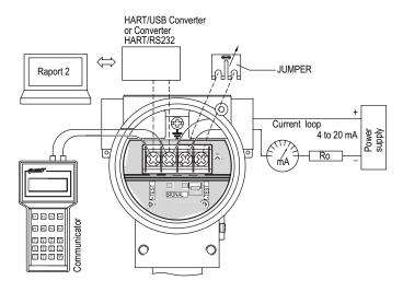
Rys. 2c Figure 3c: The link of transmitter and communicator or converter to <SIGNAL+> <TEST+> transmitter terminals in case of the resistance in current loop is smaller than 240 $\Omega$
