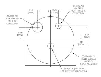
MOUNTING: The Photohelic<sup>®</sup> Switch/Gage may be either panel mounted or surface mounted.
