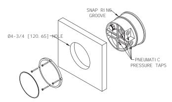
A. PANEL MOUNTING: Cut a 4-3/4" or 120mm dia. hole in panel and insert the complete unit from the front. Slip on the mounting ring and install the split snap ring in the groove on the bezel. Seat the mounting ring against the snap ring and thread the four screws through the tapped holes. Tighten screws against rear of panel.
