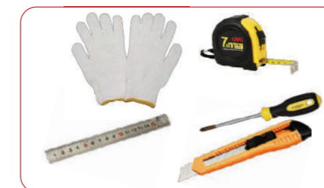
Tools set including one knife, one tape meter, one ruler, one pair of gloves and one screwdriver, for cutting rubber hose and installation of flow meter
