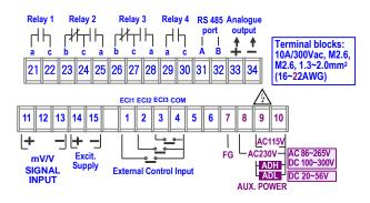
Please check the voltage of power supplied first, and then connect to the specified terminals. It is recommended that power supplied to the meter be protected by a fuse or circuit breaker.
