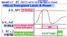
**DO function** The function has been designed not only a meter but also an I/O interface. In the case of motor control cabinet can't get the remote function. It's very easily to get the ON/OFF status of switch from CS2 series with RS485 function.
