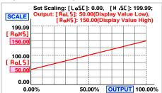
The range between [ AaHS] and [ RaLS] should be over 20% of span at least; otherwise, it will be got less resolution of analogue output.
