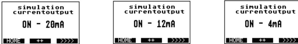
Through the use of the **++** key the output can be set to three different settings. First 20mA will be output, activating the **++** key again will set 12mA and one more activation will output 4mA. Leaving this screen will terminate the output simulation.
