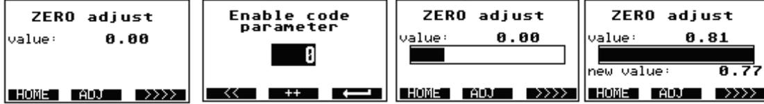
The "ZERO adjust" measurement is activated if the **ADJ** key is depressed for a period of 1.5 seconds. To perform the "ZERO adjust" it will be necessary to enter Enable code "222". To start enter a "2" using the **AAAAAA** key, then move the cursor to the left using **<<<<** key and then enter the next "2" followed by moving the cursor one last time and entering the final "2". Press the enter button **↵** to initiate "ZERO adjust".
