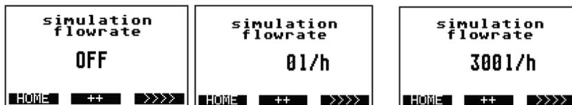
This function allows for continuous simulation of both the pulse and primary analog outputs. Using this simulation can be helpful in "dry testing" a system prior to actual use. To begin the activate the **++** key to start, the flow will read 0 gal/min. With each activation of the **++** key the flow rate will increase by 10% of Qmax. The function will be terminated by keying one additional time past the max rate.
