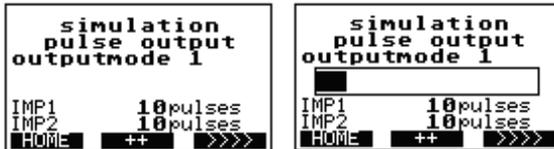
Activating the **++** key will begin the simulation. In the case of the pulse output a progress bar will display the duration of the test when complete (1 min.) A fixed amount of pulses will have been output by the meter. As with the current display this will be terminated if the screen is changed.
