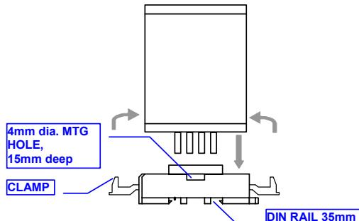
Remark: ST series has been designed in multi-output with limited terminals. Please check the output functions and specify terminals as label on product before wiring.
