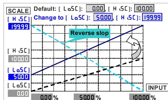
\*Lower resolution display may be caused by more narrow scale. If the [RLo] & [RH] have been changed, the [LoSC] & [HSC] will be related to the new setting of [RLo] & [RH].
