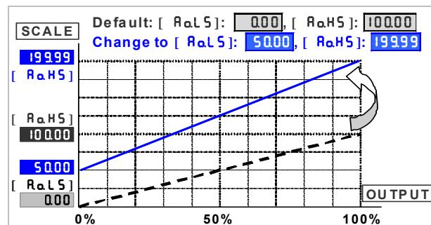
\*The interval between [RoHS] and [RoL5] should be with minimum over 20% of span; otherwise, it will reflect the less resolution of analogue output.
