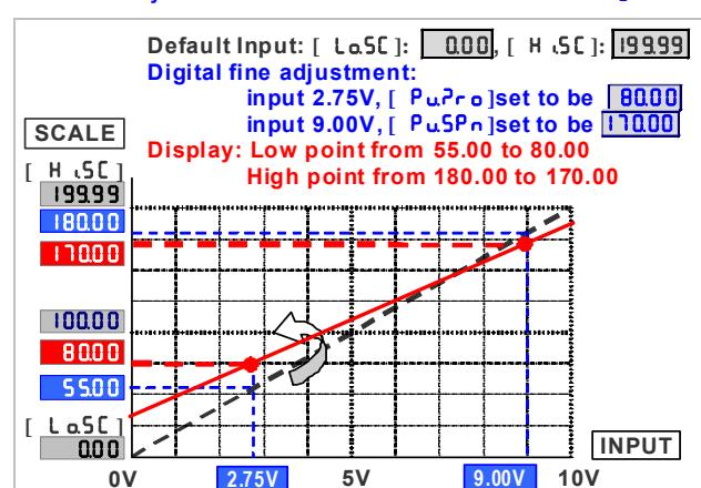
\*Please make sure that the [**Pu.Pro**] point must be less than [**Pu.SPrn**] during the process of digital fine adjustment. Generally, the interval should be over 50% of input range. If the interval is too narrow, that may be made bigger error between zero and span.
