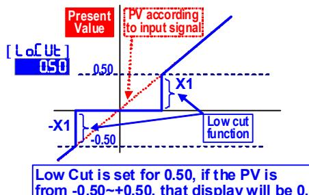
If set the negative value (X2) here to display "X2" which it expressed to be low-cut the PV that it's under the X2 setting value;
