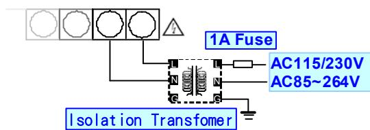
For input and RS485 wiring, Herein recommended using twin wire with shielding
