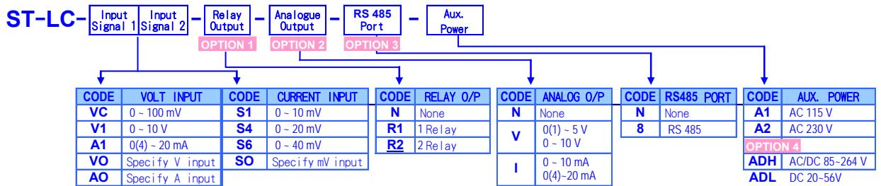
2 outputs can be specified at most for 1 Analogue > 1 RS485 及 2 Relays ;
