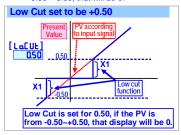
2. If set the negative value (X2) here to display "X2" which it expressed to be low-cut the PV that it's under the X2 setting
