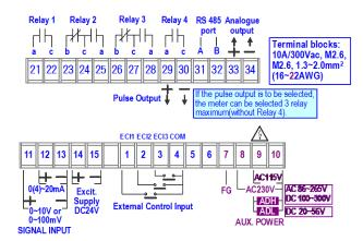
Please check the voltage of power supplied first, and then connect to the specified terminals. It is recommended that power supplied to the meter be protected by a fuse or circuit breaker.
