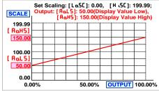
The range between [RaH5] and [RaL5] should be over 20% of span at least; otherwise, it will be got less resolution of analogue output.
