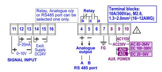
Please check the voltage of power supplied first, and then connect to the specified terminals. It is recommended that power supplied to the meter be protected by a fuse or circuit breaker.
