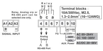
⚠ Please check the voltage of power supplied first, and then connect to the specified terminals. It is recommended that power supplied to the meter should be protected by a fuse or circuit breaker.
