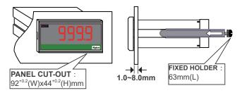
The meter should be installed in a location where it does not exceed the maximum operating temperature and provides good air circulation.
