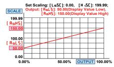
The range between [ $R_{\alpha,H}$ 5] and [ $R_{\alpha,L}$ 5] should be over 20% of span at least; otherwise, it will be got less resolution of analog output.
