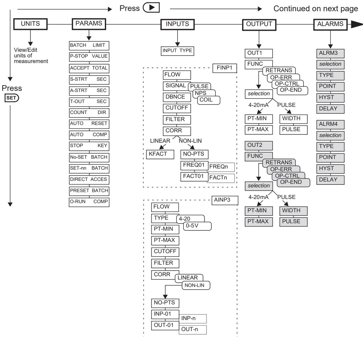
Figure 14 Calibration Menu Tree Sheet 1
