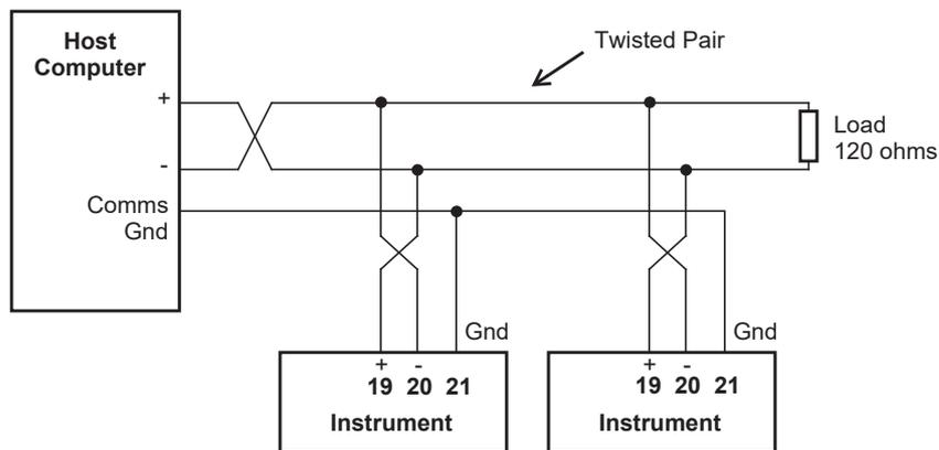
Figure 17 RS-485 Connections
