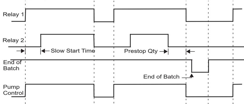
Figure 12 Batch Operation with Manual or Automatic Reset
