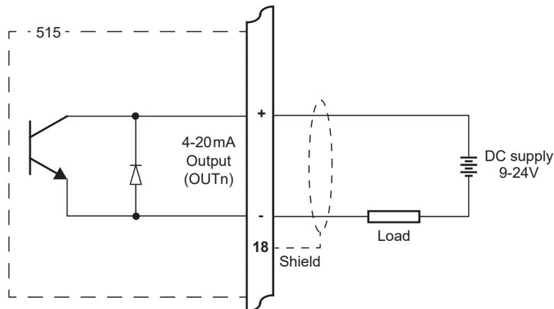
Figure 8 Output 4-20mA Connection Diagram
