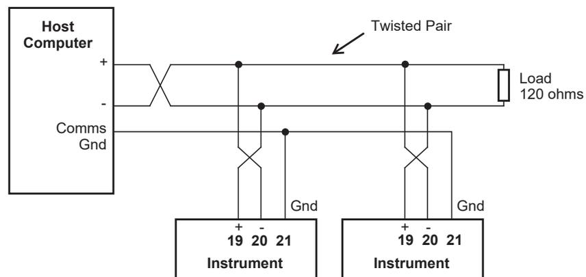
Figure 11 RS-485 Interface Connections
