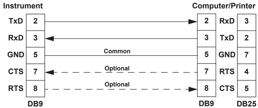
Figure 16 RS-232 Cable Connections to a Computer
